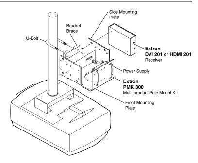
Figure 2-5 — PMK 300 projector mounting a receiver
